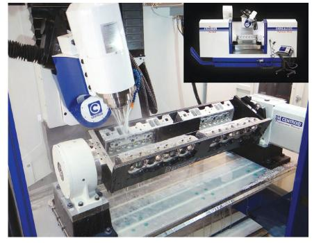
both machines along with automatic tool height measurement. Tool lengths are measured automatically.
