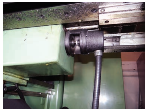
The X- and Y-axis encoders are mounted to the ends of the ballscrew and were upgraded to a high resolution unit during the upgrade.
