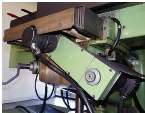
The X- and Y-axis encoders are mounted to the ends of the ballscrew and were upgraded to a high resolution unit during the upgrade.
