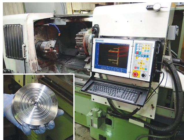
One of the regular high volume jobs at T.L. Hiner is turning compressor valve seats. Mike, the operator at T.L. Hiner, programs both Mori Seiki SL-3s with Centroid's built-in Intercon conversational programming, which prompts the operator for dimensions from the print and automatically creates the G-code to turn the part and displays the results graphically.
