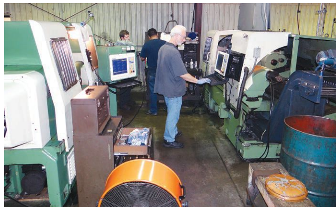
At T.L. Hiner, new Centroid T-400 CNC controls were installed on both of the Mori Seiki SL-3s in place, on the shop floor, so there was no need to move the machines for the retrofit. The two machines face each other so one operator can keep both machines running parts all day long.
