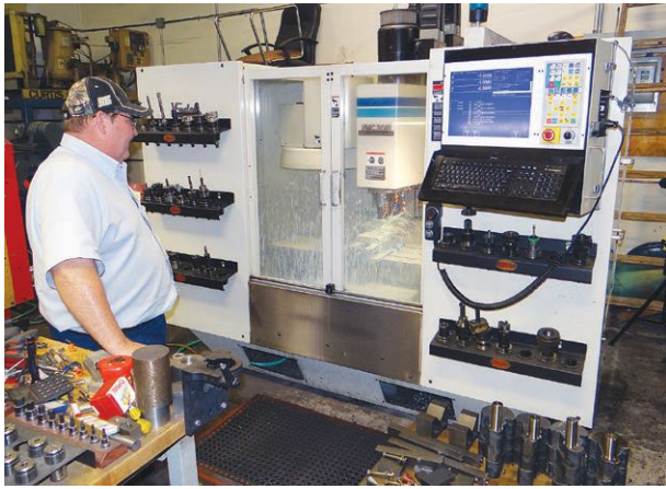
Fadal 3016 retrofitted with a Centroid M400 CNC control.
