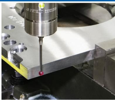
Automatic Probing cycles for every task. Inside corner, Outside corner, Bore (diameter and center location), Boss (diameter and center locations), Slot (width and center location), Web (width and center location), Single edge (X,Y,&Z). Find angles and set them square to the machine coordinate system. Produce better parts with less effort. Probing has endless applications, you'll wonder how you ever lived without this tool.
