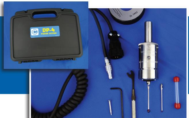
Kit contains: DP-4 or DP-7 probe, manual, external probe cable, 2.5 mm stylus, 5 mm stylus, tools, 1" standard bore gauge. Patent #6,553,682
