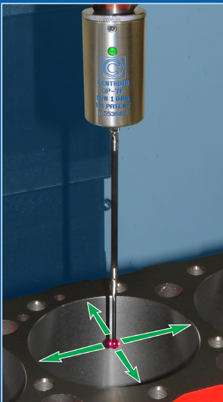
Automatic Part Setup with CNC Probing Cycles*
