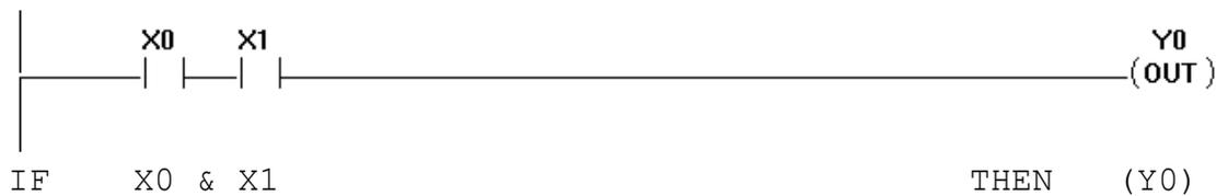
This line of program is the basic AND operation. What it means is that if X0 is on **AND** X1 is on then Y0 will be on. Otherwise, Y0 will be off.
