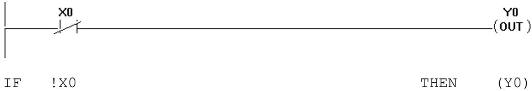
This line of program has the opposite meaning. It is an example of the NOT operation in XPLC programming. What it means is that if X0 is not off, then turn off Y0. If X0 is off, turn on Y0. Again, there are only two possibilities:
