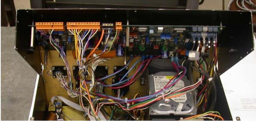
18. Double check all of the connections. Check that when the cover is closed that no wires or cables will be pinched. Be extra careful that when the cover is closed the fiber optic cables will not be pinched.
