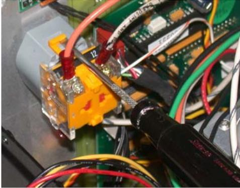
7. Remove the white wire with a black stripe that is connected between the E-stop switch block and the connector that plugs into H12 on the servo drive.
