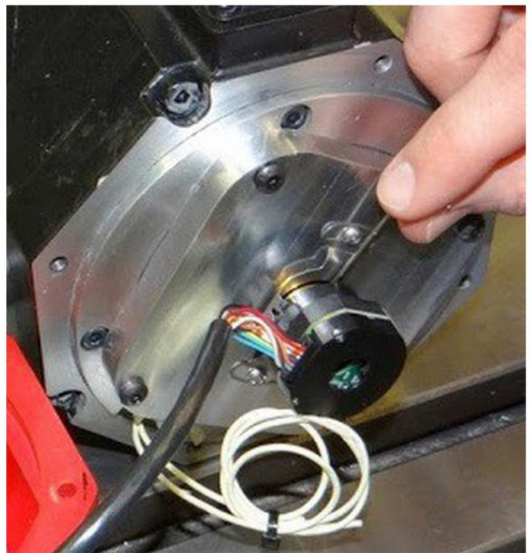
Figure 6.4.5 Encoder Alignment
