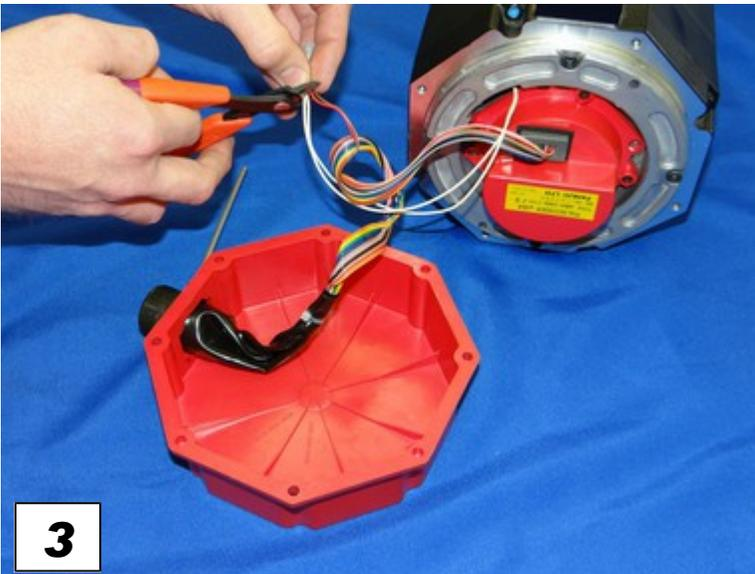
Cut the temperature sensor wire going from the motor to the pigtail connector.
