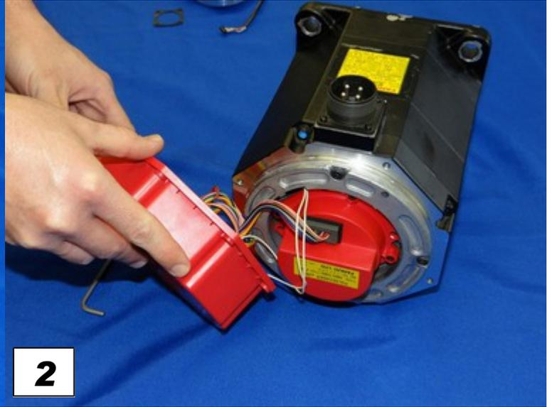
Remove the end cap and expose the pulse coder assembly.
