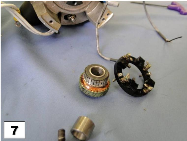
Remove the rotor of the stator of the tachogenerator.
