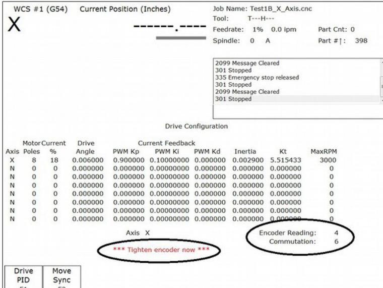
Figure 4. Encoder Alignment
