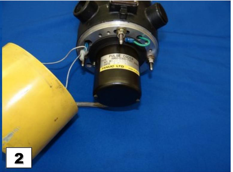
Remove the end cap to expose the pulse coder assembly.
