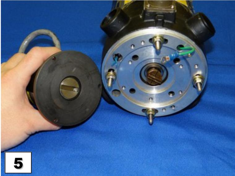
Remove the pulse coder. A brass coupling will remain on either the motor or pulse coder side.
