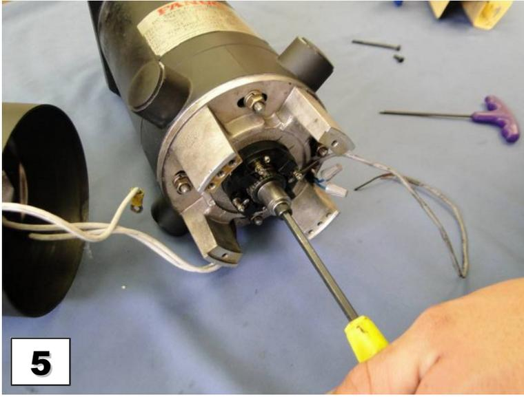
Remove the center bolt using a 5mm hex key.
