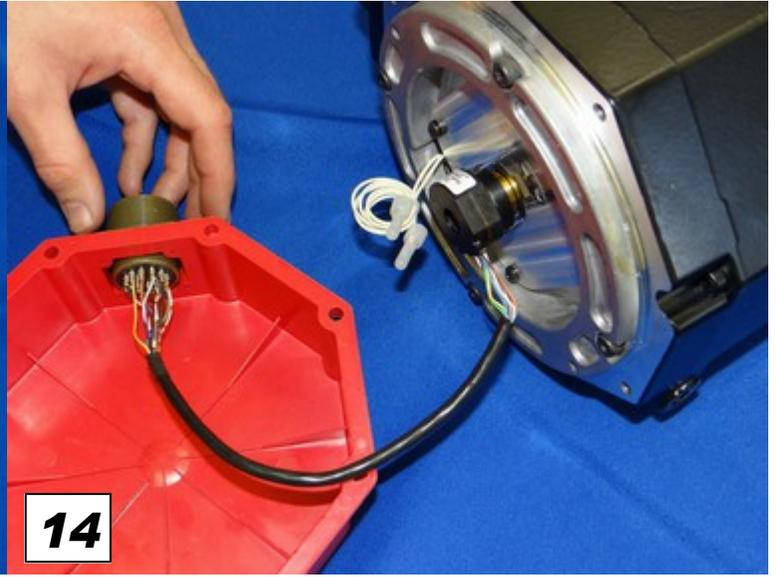
Plug the pigtail connector firmly into the encoder.
