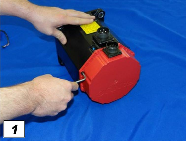
Remove the four bolts holding the red end cap in place using a hex key. Set the end cap bolts aside. You will use them again in a later step.
