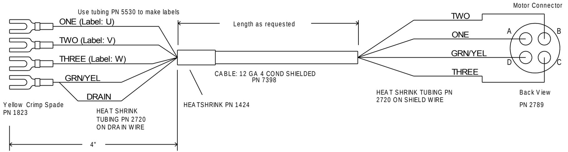
Motor cable for Fanuc Red Cap 0, 5, Beta 8is, Beta 12is, Alpha 3, Alpha 6, Yellow Cap 0M, 5M, Black Cap 0, 5, 0L, 5L, most Centroid AC motors
