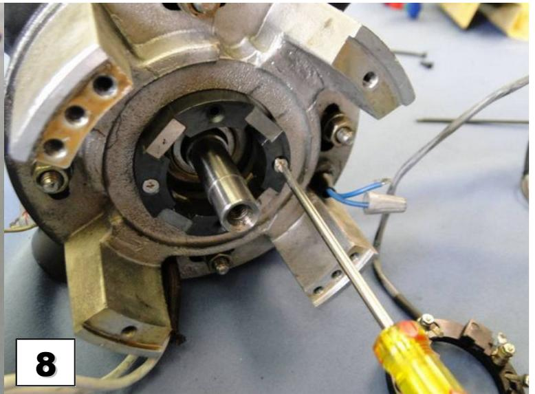
Remove the retaining screws on the inner stator with a screw driver.
