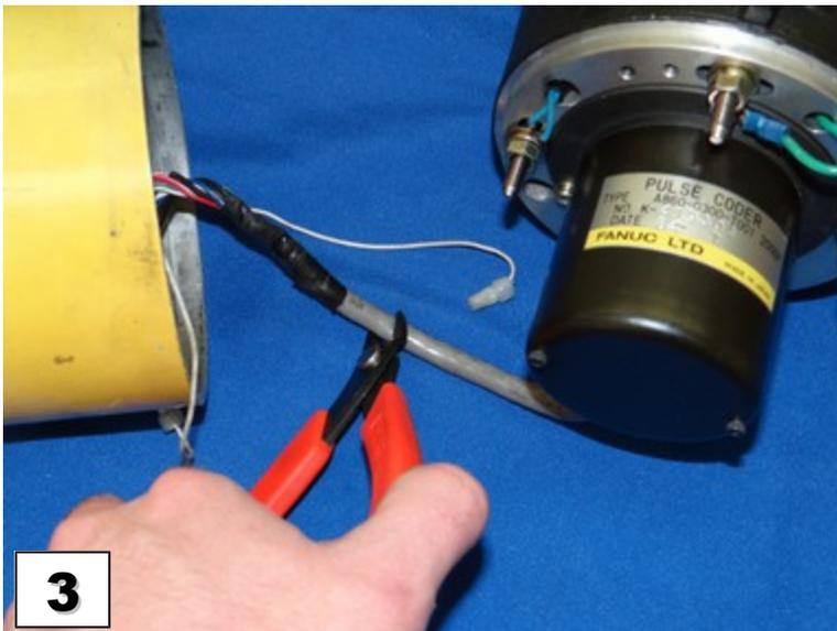
Cut the pulse coder signal cable as well as the two temperature sensor wires. **DO NOT CUT THE GROUND WIRE!**
