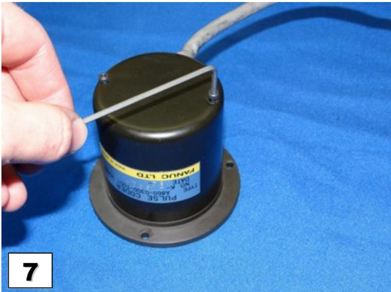
Using a hex key, remove the two encoder cover bolts.
