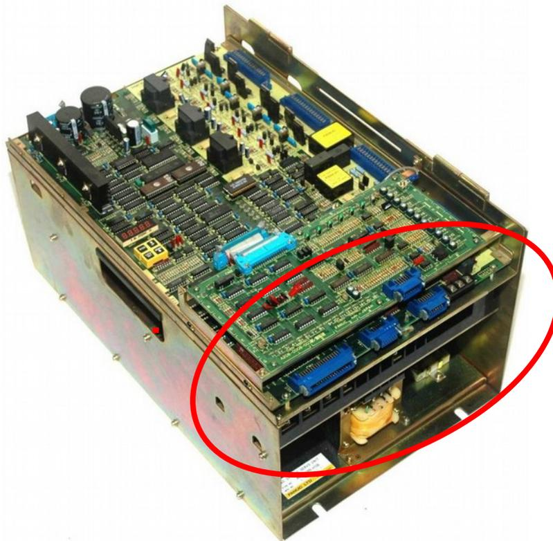
Spindle Control with the ORIENT function.
