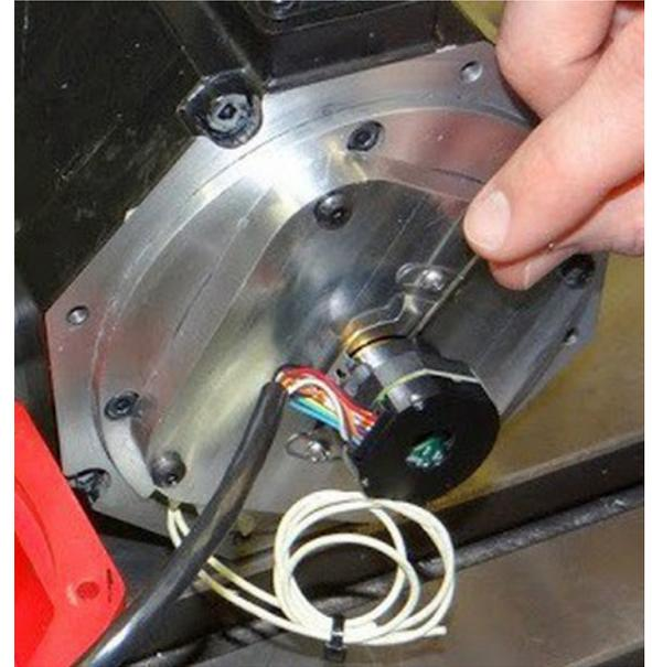
Figure 5. Encoder Collar Set Screws
