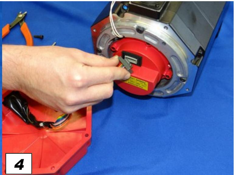
Unplug the pigtail connector from the pulse coder.
