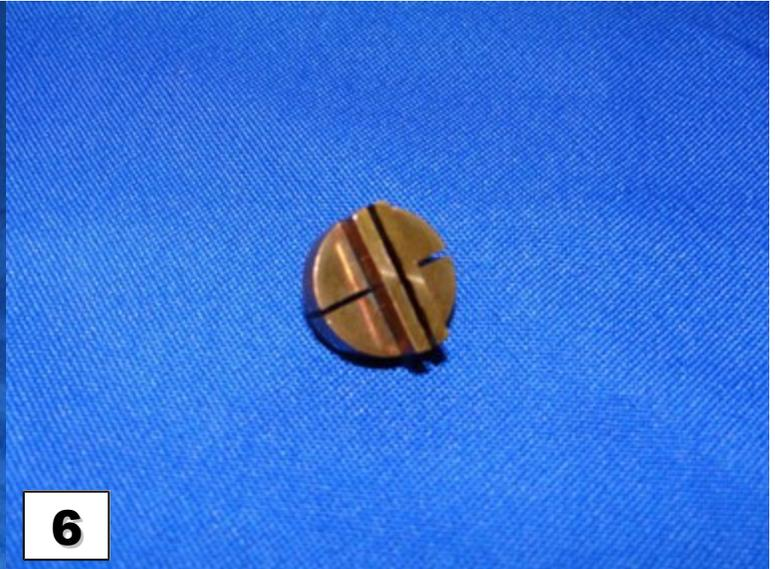
Remove and inspect the coupler. It should fit snugly into the encoder and the motor. If the coupler is worn or damaged, order a new one from Fanuc.
