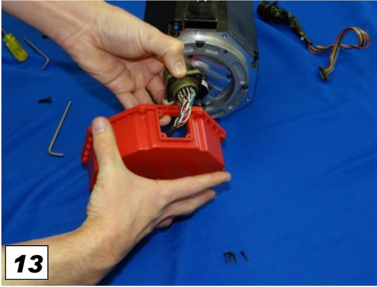
Slide the encoder pigtail with the gasket into the end cap and secure them in place with the four screws removed in step 11.
