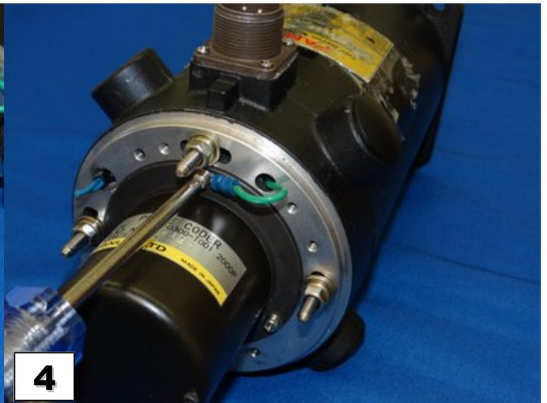
Using a Phillips screwdriver, remove the three pulse coder mounting screws. Set them aside. They will be used again in step 21.
