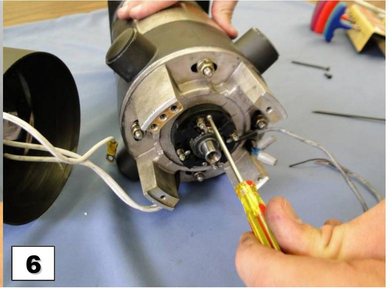
Remove the retaining screws on the outer stator with a Phillips screwdriver.
