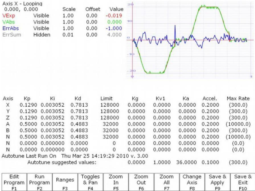
The colors of the text on the top left match the colors of the graphs on the right. For example, if you have a V abs value written in blue in the top left, the graph for V abs will be displayed on blue in the top right. For the rest of the tuning procedure when referring to motor velocity, we are referring to the **V Abs** value and the corresponding graph. When referring to position error, we are referring to the **Err Abs** value and the corresponding graph
