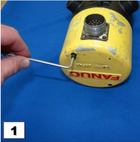
Remove the two bolts holding the black end cap in place using a 3mm hex key. Set aside the end cap bolts. You will use them again in a later step.
