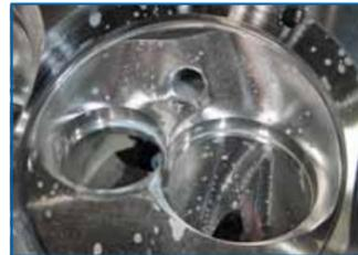
Machine perfect combustion chambers every time. By combining CENTROID's smooth motion control and built-in digitizing software with Mastercam's advanced toolpaths, you can easily reproduce your hand-ported designs with results superior to other methods and machines.
