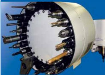
Equipped with a 24 pocket Automatic Swing Arm Tool Changer the A560 holds enough tools for both cylinder head and block work. Tool changes are fully automatic, taking just a few seconds. Tool changer is located up and out of the way of the work envelope of the machine and does not take up any work space.
