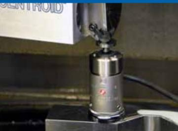
Eliminates operator error and increases accuracy. Automatic Tool Length measurement, takes the guess work and labor out of setting up tools. Menu driven, push button measurement only takes a few seconds for each tool. More accurate and much faster than setting tools by hand.
