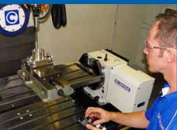
Bolt-on T-slot table to hold any part. Converts machine into a general machining center. Allows you to quickly switch from heads or blocks to general machining. T-Slot table accepts: parts, vises, custom fixtures, & cylinder heads with standard hardware.
