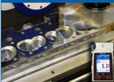
Achieve low RA's with CENTROID's own surfacing tooling. Designed and manufactured in-house specifically for cylinder head and block surfacing. T-Slot table accepts cylinder heads for surfacing.
