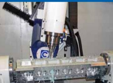
High Torque 27HP, 40 taper spindle delivers much more low end than the other guys. The A560 can easily machine a large variety of materials providing superior surface finishes while delivering the low end torque necessary for drilling, tapping & roughing out material. 100% duty cycle spindle operation.
