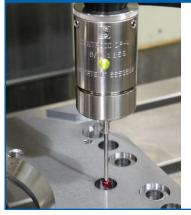
Quickly and accurately find zero points on a vise, fixture or part. Eliminate operator error when setting zero points, finding edges, or center locations of bosses or bores, slots and webs.
