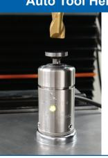
Automatic Tool Height Measurement.An invaluable tool for a wide variety of CNC machines. Quickly, easily and accurately setup tool heights in the tool library with a push of a button
