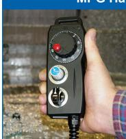
Jog an axis with a MPG handwheel. Selectable x1, x10, x100 movement per increment. .0001" per increment is the finest increment. Great for touching off and setting up tools and part zero positions.
