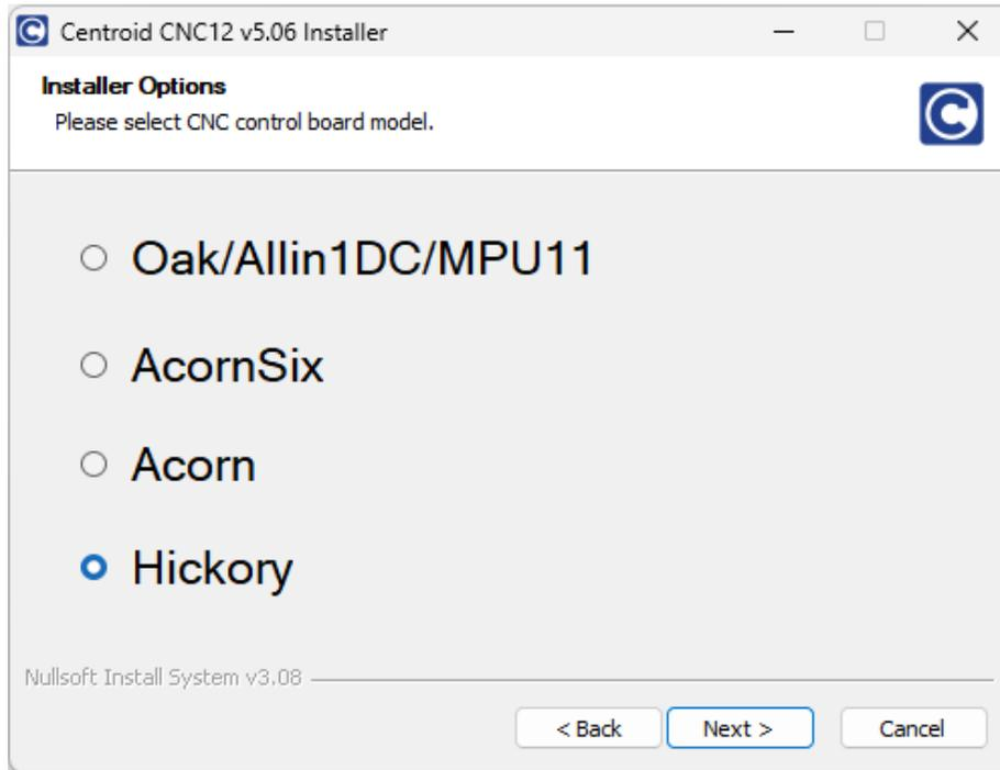
9. Select which CNC software component is correct for your machine. Select “Next” to continue.
