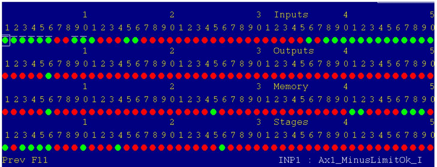
4. If the limits are still inverted from bench testing, there will be a bar above inputs 1-6. Remove the inversion from these inputs by pressing <Ctrl + Alt + i> for each input 1-6.
