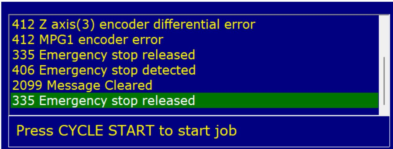
Notice that as you toggle the E-Stop input to red, “406 Emergency stop detected” is displayed in the status window, followed by “2099 Message Cleared.” When the E-Stop input is toggled green, notice how “335 Emergency stop released” is displayed.
