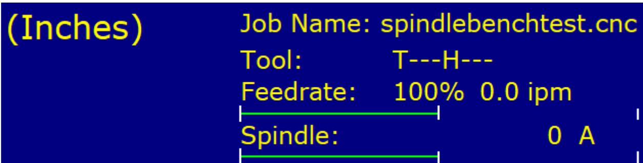
3. **Testing the analog output.** Hickory provides 0 to +10VDC analog output for the purpose of programmable spindle speed control using a VFD (variable frequency drive). The default maximum spindle speed specified in the Control Configuration is 3000rpm. This configures the control to scale the 0 to +10VDC signal from 0 to 3000rpm. A spindle speed command of S1500 should therefore output +5VDC, a command of S1000 should output +3.33VDC, and so on.
