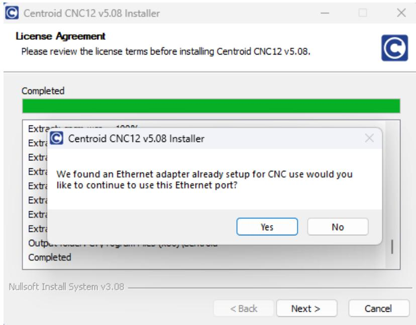
2. If the Ethernet Adapter has not yet been set up for CNC control, you will see the screen below. Select the Ethernet option to automatically configure the IP address for CNC use and click “Next”. **DO NOT** select the Wi-Fi option.
