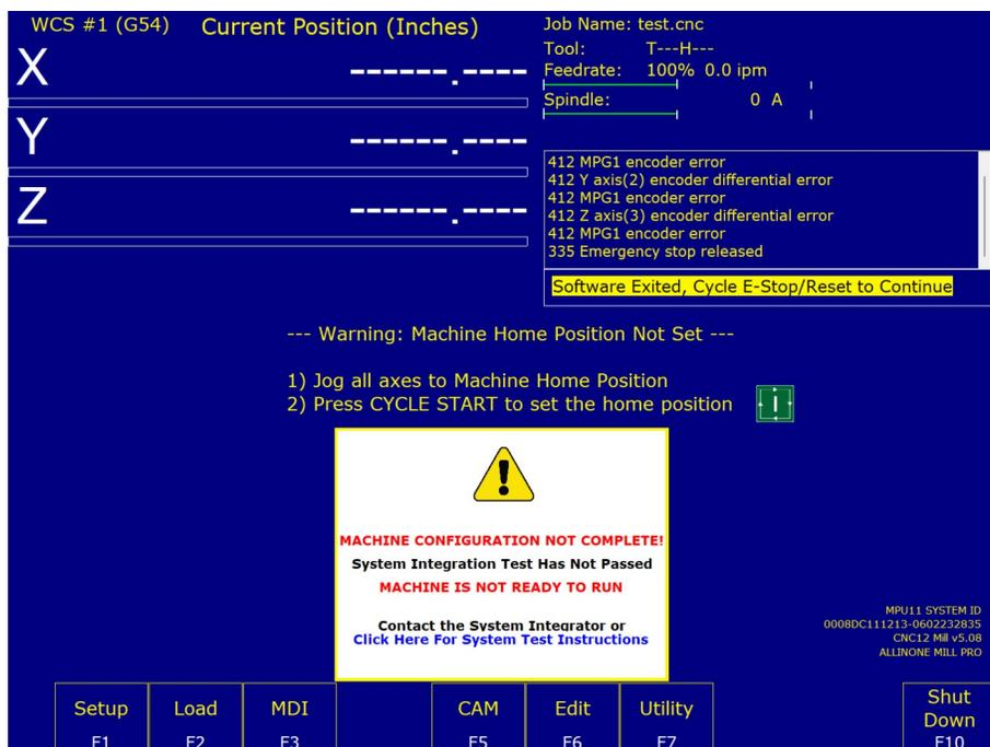
To clear a stop fault, press <Alt + i> to bring up the real-time I/O screen. Use the arrow keys to select “INP 11: EstopOK\_I” as shown below. Press <Ctrl + Alt + i> to toggle the E-Stop input so that it turns red, then again so that it turns back to green.
