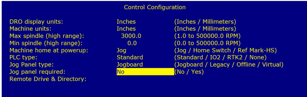
After saving, press **ESC** to go back to the Main Screen. Press **F10-Shutdown** → **F2-Power Off**. After the computer shuts down, cut the power to the Hickory and the PC via switching off your outlet strip. Wait 30 seconds and power everything back up.
