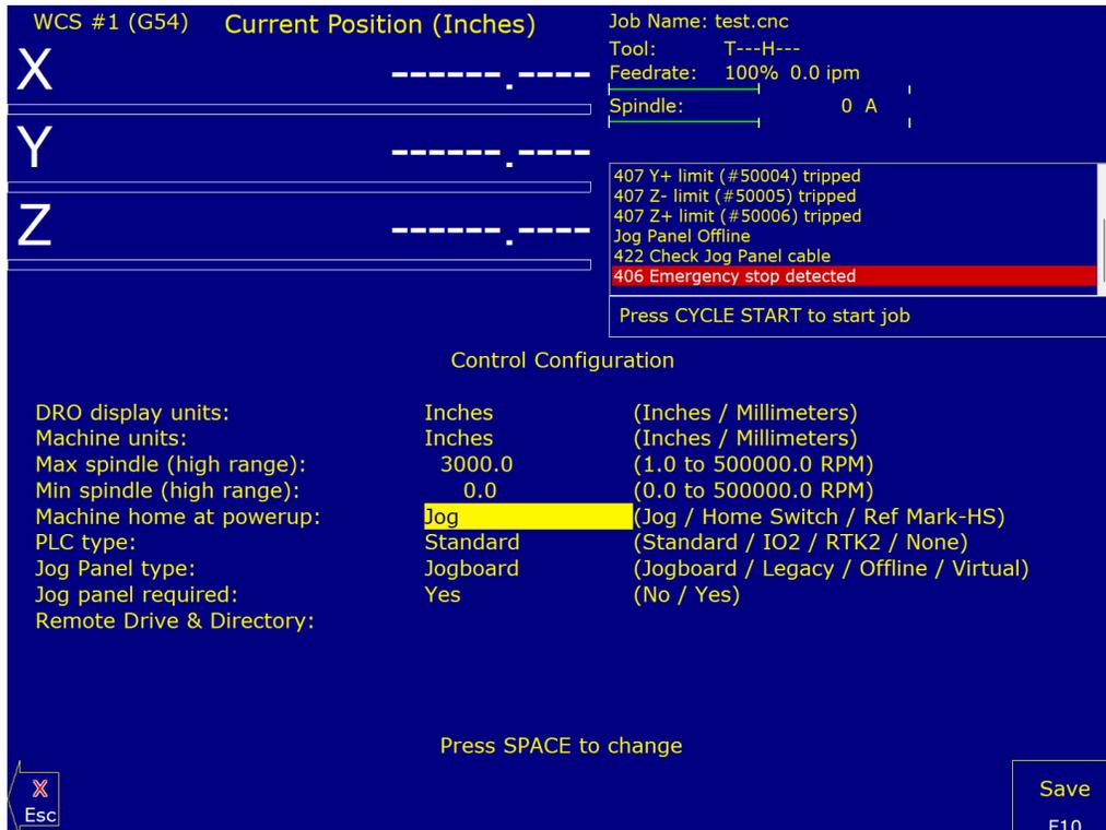
2. **Disable Jog Panel Communication Faults** (If you have a jog panel or pendant, connect it and skip this step.) Disable Jog Panel communication faults. Use the arrow keys to select “Jog Panel Required” in the Control Configuration and press the space bar to toggle to “No”. Press **F10-Save**.
