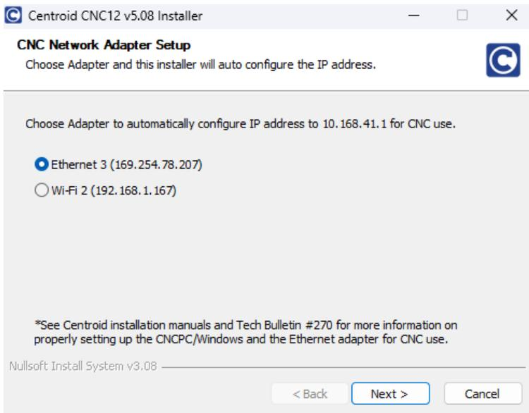
3. If the Network Adapter Setup screen does not show an Ethernet option, that means that the installer does not detect the CNC control board Ethernet connection to the PC. **If you see this screen STOP, select "Cancel"**, and ensure that the control board is powered on and connected to the PC via Ethernet. Then retry the installation. If the issue persists, go back to [Section 3.1](#) and check the Windows 10/11 configurations are setup properly for CNC control use.
