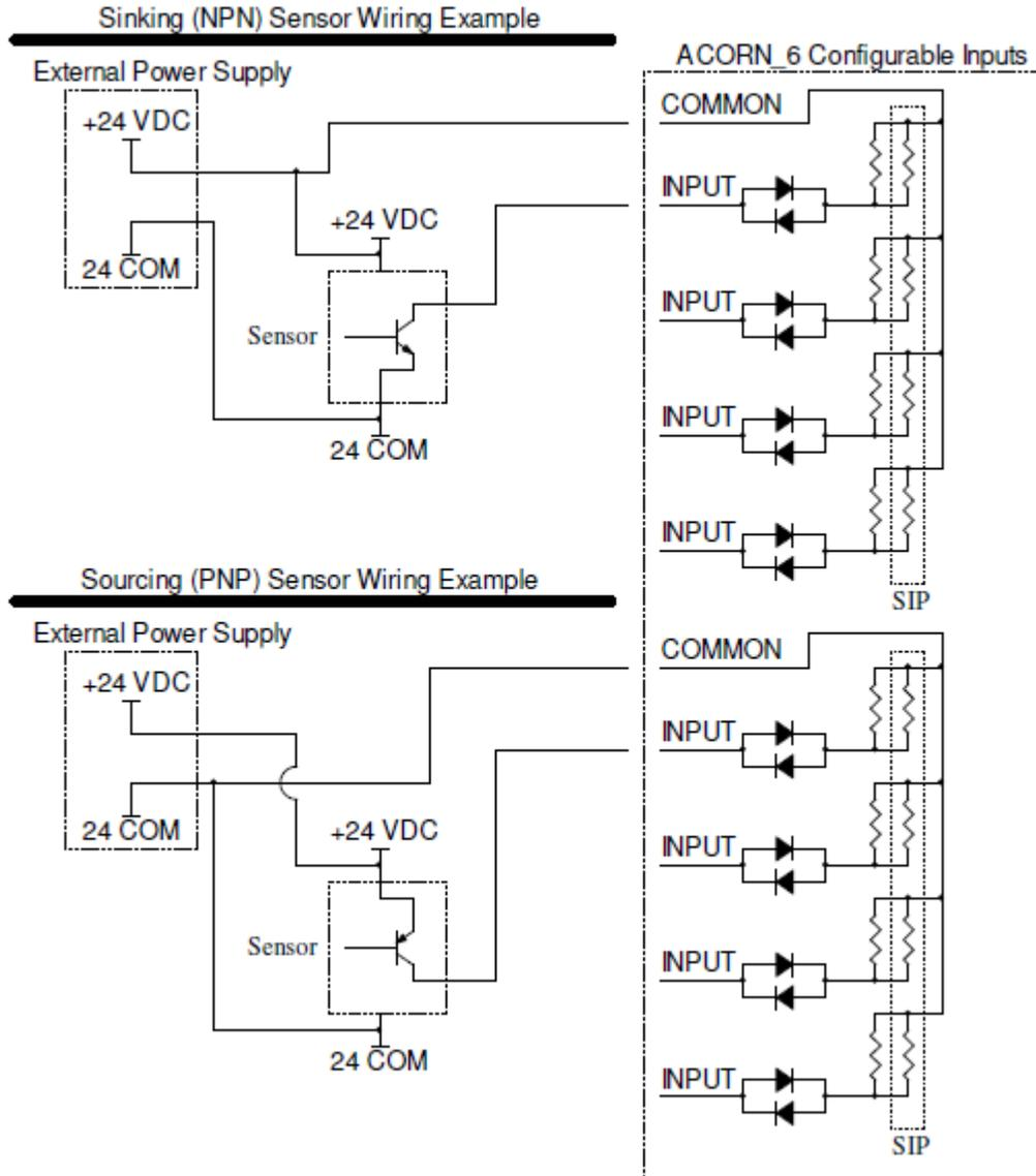
Voltages can be selected by installing the appropriate SIP. Without a SIP installed (default configuration when shipped from Centroid) the voltage is set to 24V. Optional SIPs can be installed to use 12V or 5V input voltage.
