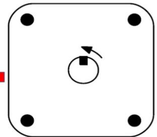
Rotating the shaft counter clockwise increases the value in the “Abs Pos” field of the PID Menu.
