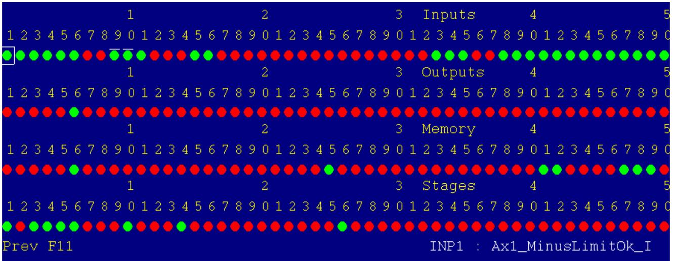
6. Confirm that the correct input turns red when the switches are manually tripped.
