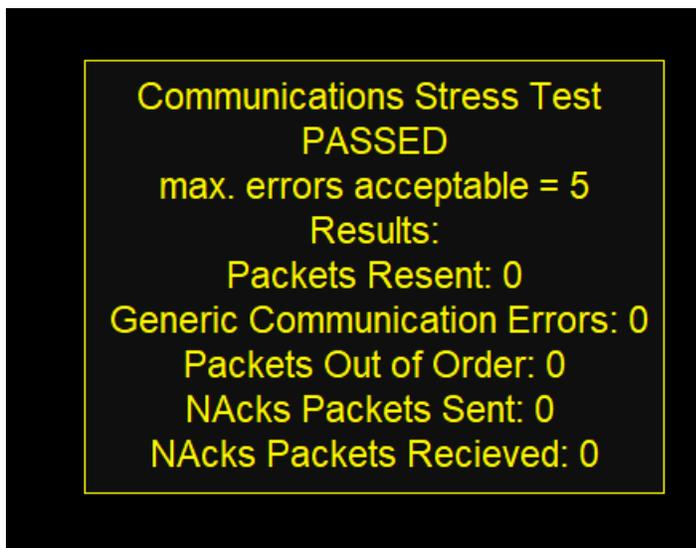
If the stress test fails, that indicates that there are major communication issues between the PC and the controller which can result in a non-functioning machine and potentially a hazardous working environment.
