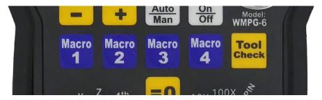
The WMPG Macro buttons are preassigned to the following user editable macros located in the cnc12 main directory (starting with cnc12 v5.4 mill = c:cncm, lathe = c:cnct, router = cncr, plasma = c:\cncp, laser = c:\cncl )
