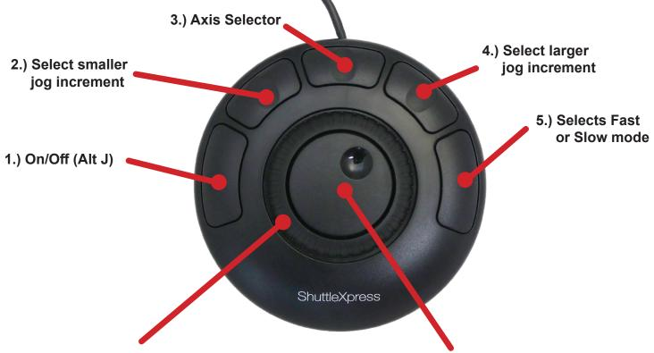
7.) The Outer Jog Wheel jogs any axis continuously. The further you rotate the wheel the faster the axis jogs. Jog speed override increments are 10%, 35%, 75%, 100%, 135%, 175% and 200% of the set fast or slow jog value. Feed rate override percentage returns to 100% when the outer wheel returns to center. (Note: If you have parameter 39 set to limit the feed rate override percentage, the outer wheel will not exceed that limit)
