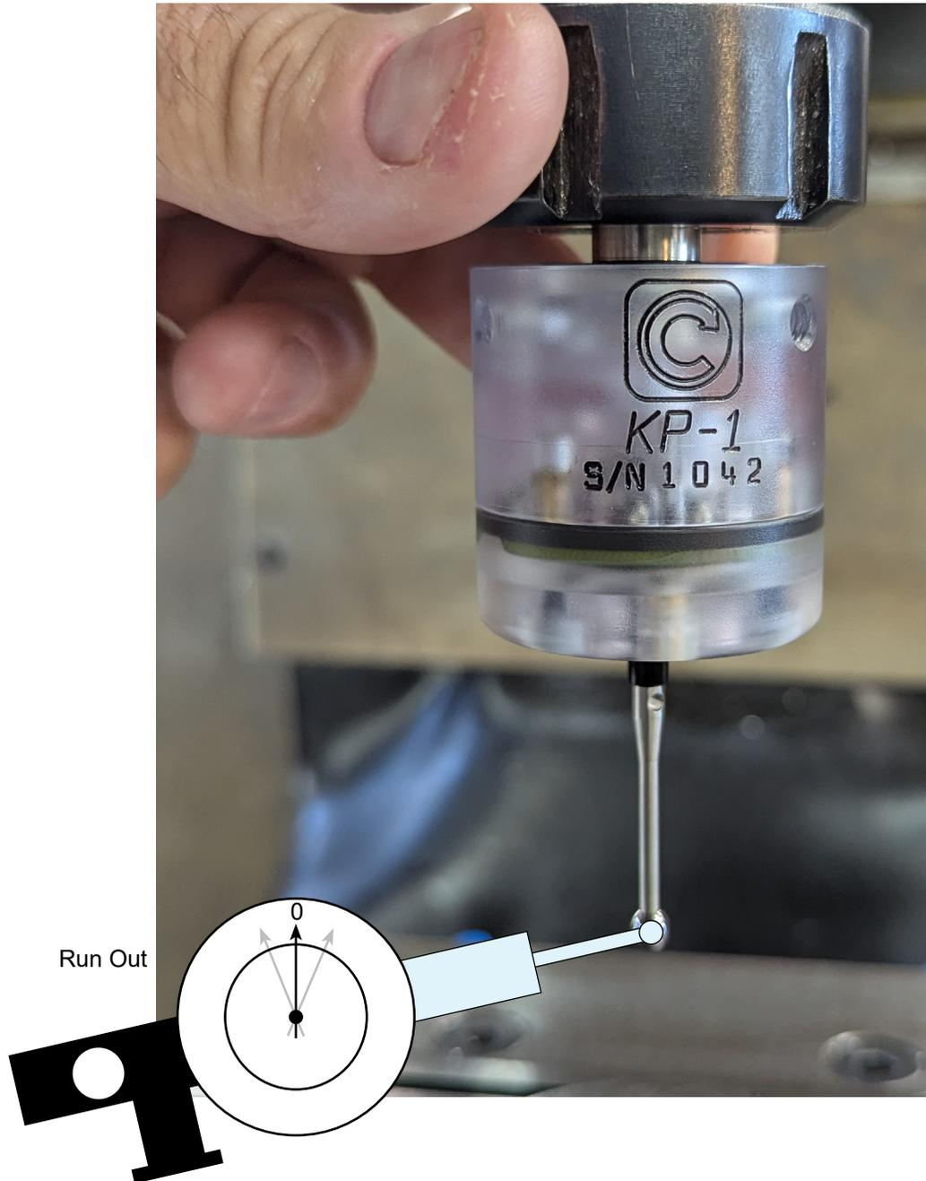
STEP 3: Rotate the spindle by hand (without touching the probe) so that the probe spins through a full 360 degrees and watch the dial indicator to locate the high and low run-out rotation positions of the stylus. Adjust the dial indicator so that the entire run-out of the tip can be seen on the dial. If the run-out exceeds the range of the dial then begin at the highest point of the run-out and set the dial indicator so it is at the limit of its range at this point.
