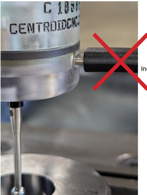
Incorrect, probe cable connector is not fully seated.
