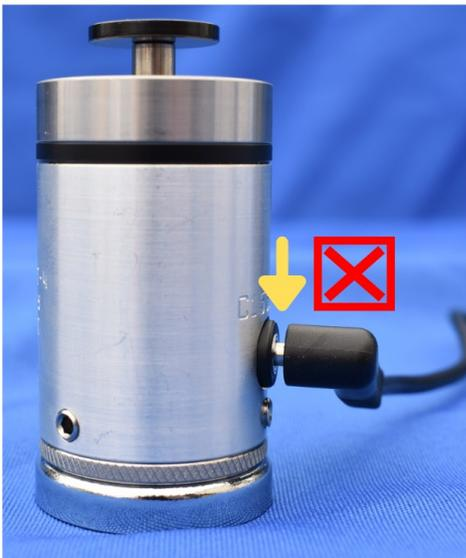
Incorrect, TT-4 cable connector is not fully seated
