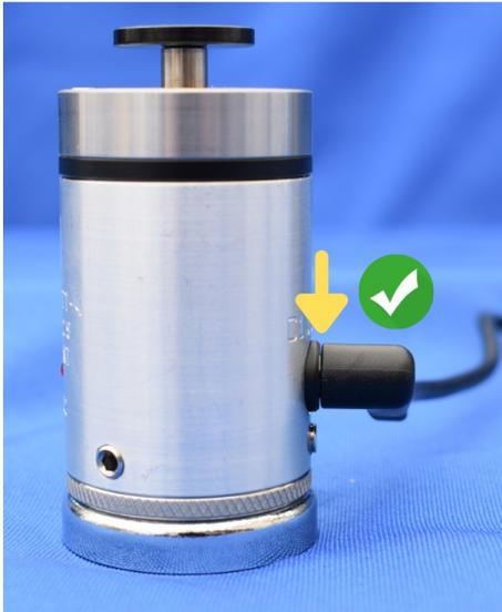
Correct! TT-4 Cable connector is fully seated
