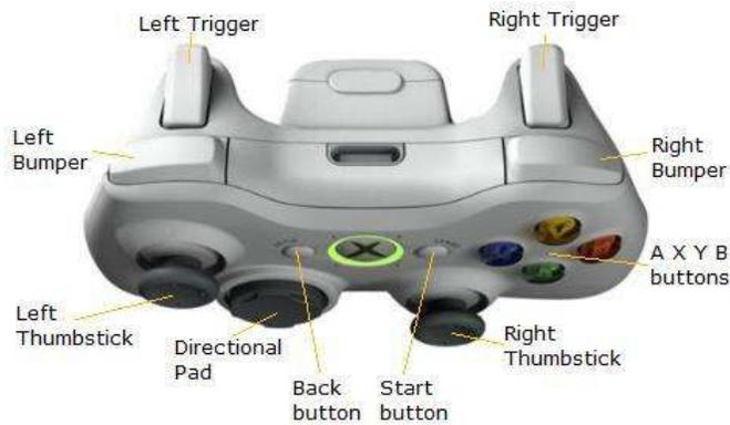
On the top edge of the XBC are two triggers which can't be seen from the front. I have assigned the Left Trigger (LT) the key Del (Delete) and the Right Trigger (RT) the key Ins (Insert).
