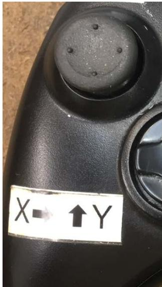
For example, I have chosen to control my X axis with the upper left joy stick. Moving it to the right moves the cutter with respect to the table to the right. Moving the stick to the left moves the cutter in the opposite direction. Additionally, I set up this joy stick to control my Y axis in a similar fashion.
