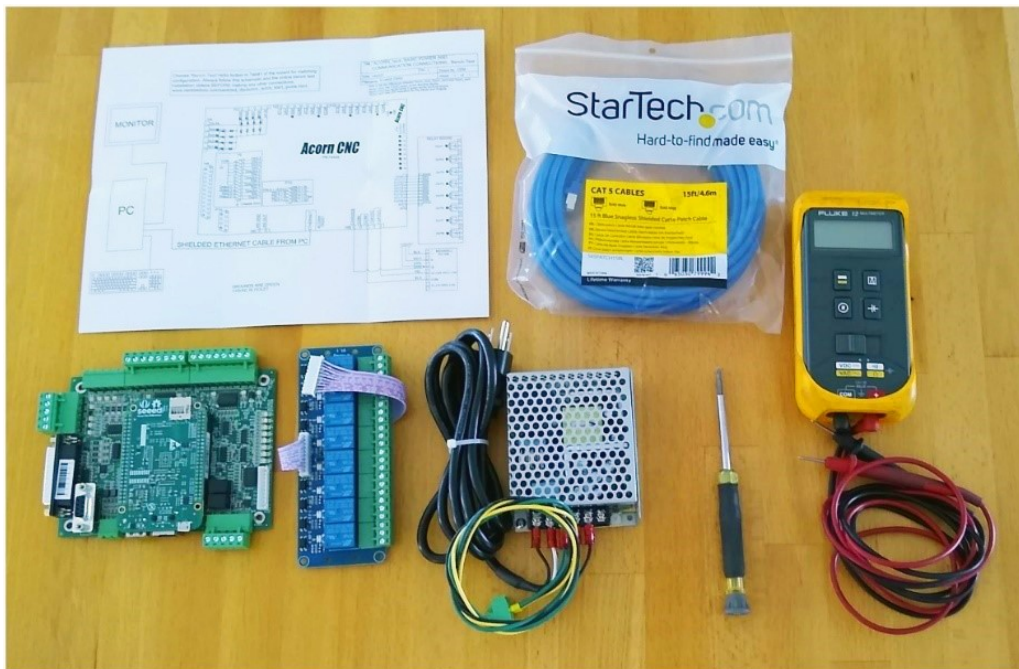
Items needed to setup the Acorn controller for bench testing
