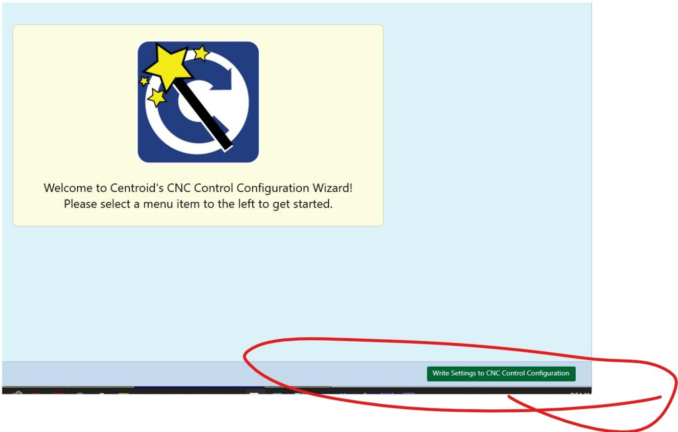
This is a critical step as the Wizard will create a new PLC program that works with v4.80 based on the previous Wizard settings avoiding the having to hand adjust all the settings in the Wizard and enabling new features not available in the previous version.
