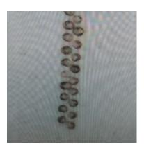
As you can see the machine has backlash in this axis and is loosing motion when changing directions. Since each "dot" is 0.006 inches long we can make an educated guess at the backlash adjustment need to align the "dot"
