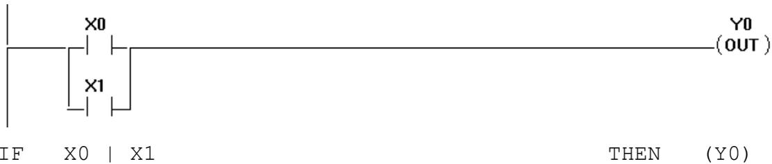
This is the basic OR operation. What it means is that if X0 **OR** X1 is on, then Y0 will be on. Otherwise, Y0 will be off.
