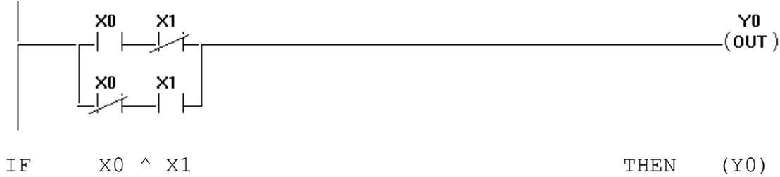
This example shows the XOR operation. What it means is that if one of X0 or X1 is on (1), but not both, then Y0 will be turned on (set to 1). Otherwise, Y0 will be off (reset to 0). The truth table is below. Another way of stating this is that if both of the inputs do not have the same value, then the result is true.
