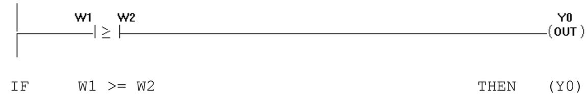
The above examples demonstrate comparisons between integer type operands. What they mean is that if the comparison is true, then turn on Y0. Otherwise, turn it off. In the first program line above, if W1 = 3 and W2 = 4, then Y0 would be turned off.
