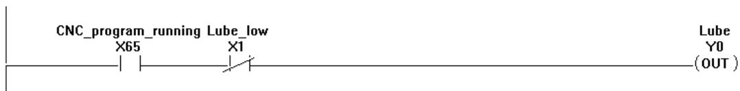
Note here that an “IF” is represented graphically as |-- , with THEN being interpreted as a coil connection at the end –(.
