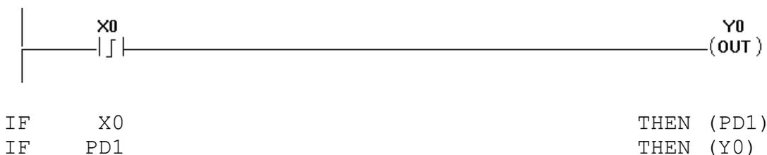
This example demonstrates the use of a positive differential, or rising edge one-shot type of contact. What it means is that if X0 is off one pass and then on the next pass, then Y0 will be turned on for one pass. Perhaps a timing diagram can better show this.
