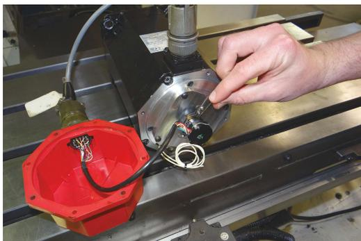
Here, a procedure is being performed to align a new Centroid encoder to a machine's original FANUC red cap servomotor. Using an original servomotor that is still in good condition not only lowers retrofit cost, but also eliminates the need to create adaptor plates and buy new pulleys, couplers or gears (or modify existing ones). These costs can be particularly significant for large machines.
