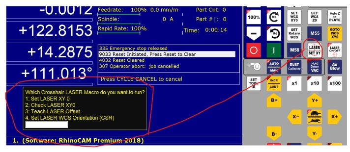
30. Router CNC12 VCP now has a "Set Tool #" button to make it easy to set the current tool number for router users that don't use the "mill style" part Z zero menu.
