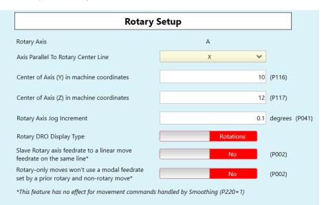
M151 now also works with any rotary axis. (previously only available in CNC12 Lathe for C axes) M151 when used with a Rotary axis acts as a "DRO unwind". M151/A will reset the DRO to a value between 0-360 degrees. So for instance if the Rotary axis has "wound up" past 11 turns and is at 11R121.462 (121.462 degrees)
