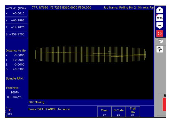
28. Jogging speed override now uses Feed Override percentage for speed calculation instead of Rapid Override speed percentage.
