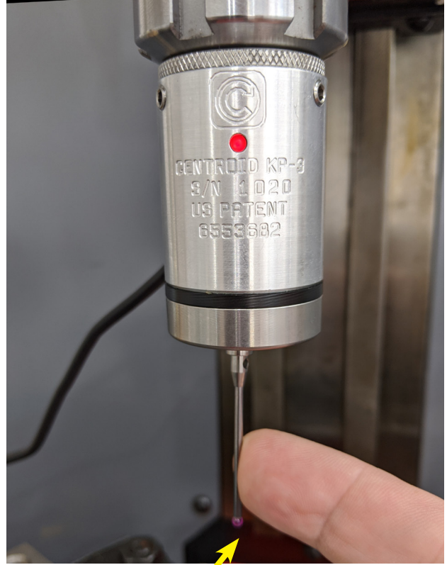
Gently trigger with finger while running a probing cycle in air to test probe before using the Touch Probe
