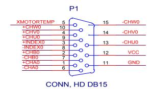
**Spindle Encoder Input** This input does not require commutation channel and is compatable to previous wiring.
