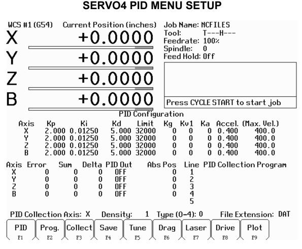
F1 PID Key will enable you to adjust the above parameters. Ka should be left at zero, while the Kg and the Kv1 may be set by observing the PID Out while the axis is at rest and during a slow jog respectively.
