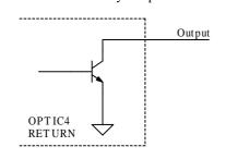
OPTIC4 Internal Circuitry E-stop / Fault Relay Output E-stop Contact 1 E-stop Contact 2
