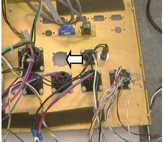
12. Remove the cover plate from the CPU7 card. After marking the Jog panel cable connector to make sure it will be reconnected correctly, disconnect the jog panel cable. After making sure that the TXS, CKS and RXS fiber optic cables are clearly marked, remove the fiber optic cables. The DATA and SYNC fibers will not be reused and should be separated from the other 3 fibers. Remove the CPU7 card.
