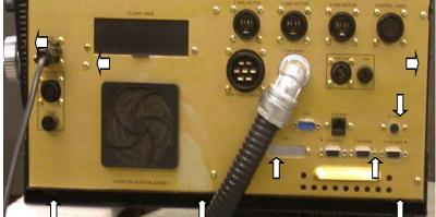
16. Connect the wires from the conduit to the correct locations. (See schematic drawing) Connect the 4<sup>th</sup> axis encoder cable to the 4<sup>th</sup> axis ribbon cable DB9 connector. The cables and wires should also be bundled and routed so that nothing is pinched or stretched. (Use the drive for reference when routing cables.)
