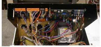
6. With the top cover and drive removed remove the switch block from the back of the E-stop switch. Disconnect the cable for the MPG connector.
