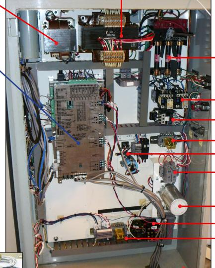
Main 3 phase fuses (use a VFD to run on single phase)
