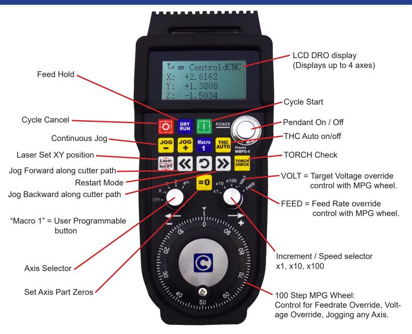
Take the control to where the work is! A game changing tool, the Centroid Wireless MPG Control Pendant allows the operator to conveniently and precisely set up jobs and tools remotely. No software drivers to install. Plug and Play with Centroid CNC12 CNC software, just plug in the included USB transmitter/receiver and start using it!
